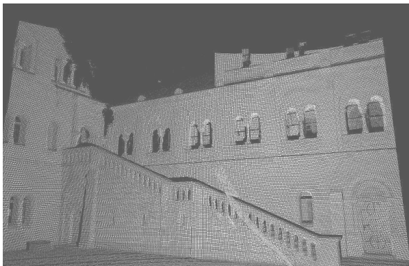
Figure 4: 3D Point cloud by IMAGER 5003
