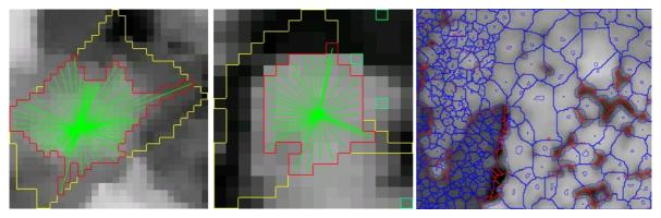
Figure 4: **Ray-algorithm** - 4a,b) show two examples, where the regions created by the pouring algorithm are reduced, based on a slope criteria. 4c) shows the final result after the ray algorithm. The blue border lines show the new corrected and the red ones the part of the border lines, which have been calculated by the merging algorithm.
