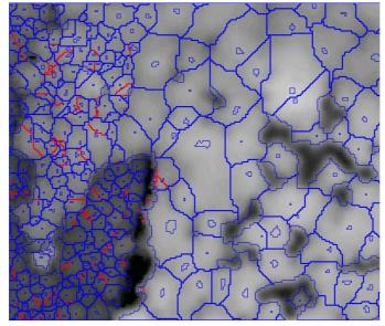
Figure 3: **Merging Algorithm** - The regions calculated by the pouring algorithm are changed. The blue border lines show the corrected and the red ones the part of the border lines, which have been originally calculated by the pouring algorithm.
