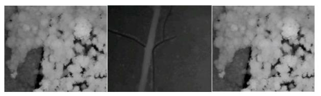
Figures 1: 1a) shows the **DSM** from the test site West of Freiburg (South Germany); 1b) shows the **DTM** and 1c) shows the normalised DSM (**nDSM**), calculated by subtracting the DTM from the DSM. Tree heights can by measured directly in this model.
