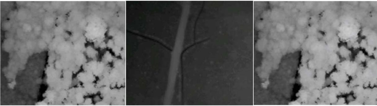
Figures 1: 1a) shows the **DSM** from the test site West of Freiburg (South Germany); 1b) shows the **DTM** and 1c) shows the normalised DSM (**nDSM**), calculated by subtracting the DTM from the DSM. Tree heights can be measured directly in this model.
