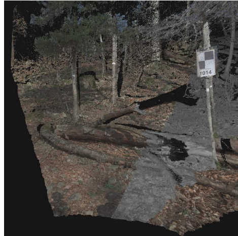
Figure 12: The figure shows the 3D point cloud of a group of trees in a forest, partially combined with colour information. There remain dark shadows, as the data acquisition was taken from just one viewpoint.
