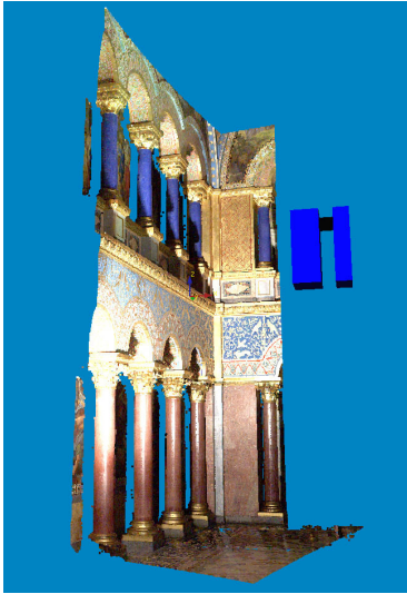
Figure 10: The figure shows a part of the drawhall of castle Neuschwanstein as colored 3D point cloud.
