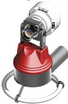
Figure 7: The figure shows the high resolution DLR line scan camera.
