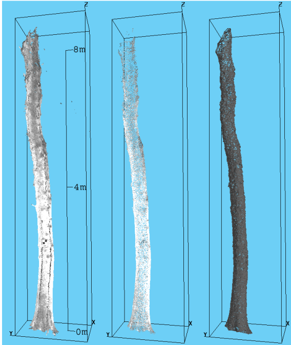
Figure 4. Tree point triangulation by power crust algorithms. Left is the points cloud of a oak tree with 800,000 points. In the middle the reduced point cloud with 50,000 scan points. Right the generated triangulation.
